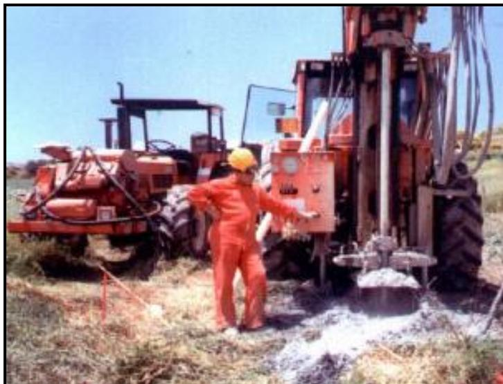
**Figura 2.3.4.2b Gruppo di Perforazione Mini L.I.A.**
