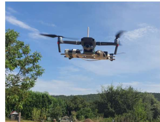
UAV DJI Mavic 2 with LoRa gateway onboard
