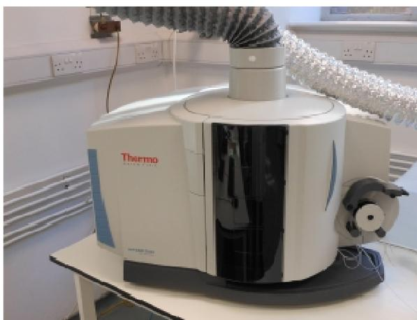
Figura 2.5 - Thermo iCap 6500 Duo ICP-AES
